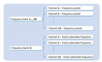
Each of the channels in the frequency banks "1" to "20" has been factory-preset to a fixed transmission frequency (frequency preset). The factory-preset frequencies within one frequency bank are intermodulation-free. These frequencies cannot be changed.
