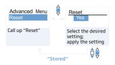
When resetting the radio microphone, only the selected settings for the pilot tone and for the frequency bank " $\cup$ " remain unchanged.
